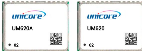
Figure 1-1 UM620 Series Modules (Left: Automotive; Right: Industrial)
